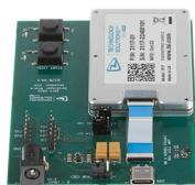
RAIN Development Board including module
